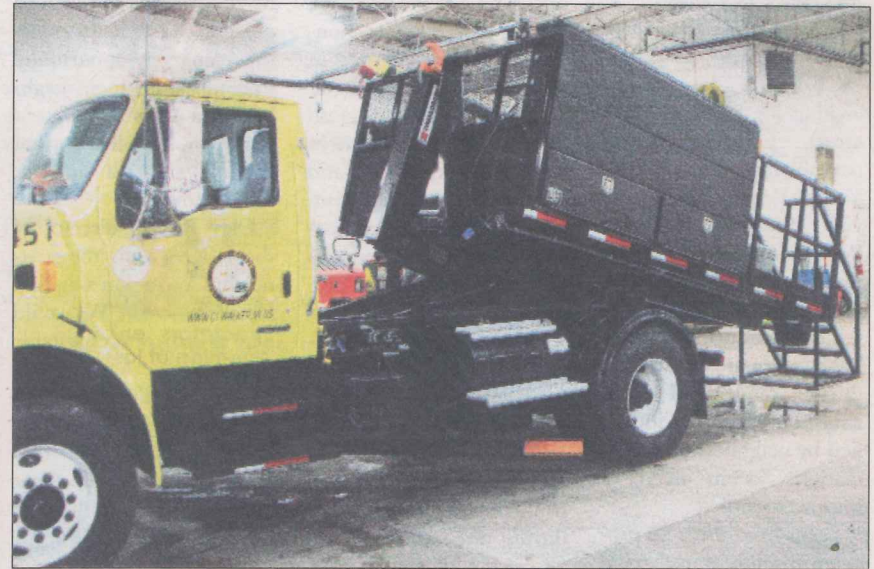
This former salt truck has been converted to now be able to change from a salt truck to a sign platform truck to any number of uses in a matter of minutes.
